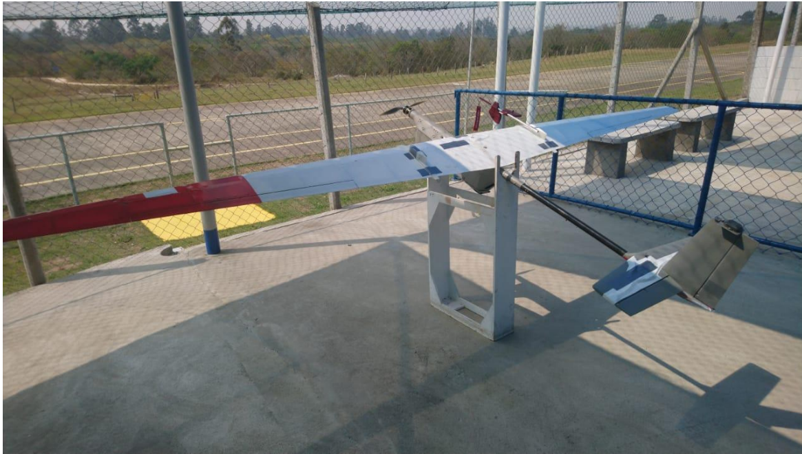
Figure 1 – EOLO aircraft with flexible wings manufactured by FT Sistemas in 2018
